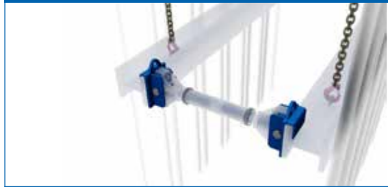
Mounting and extending the spindles on the walers
