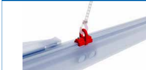
Transporting slide rails and fitting to frames
