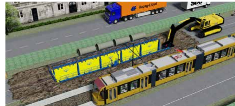
Fig 1: Loads on and in the ground
